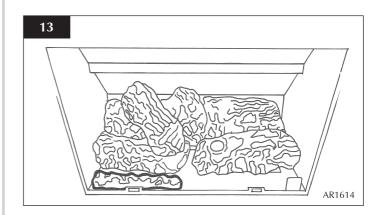
5.4 Place the second ash panel to the right of the first, with the pointed end of the panel fitting into the V shape. This panel should locate on the screw holes of the burner skin. Ensure that both logs are horizontal to the burner ports.
